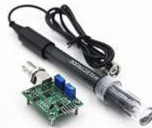
**Gambar 3.** Sensor pH Air
