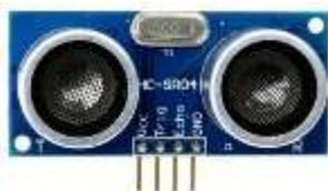
Gambar 5. Sensor Ultrasonik HC-SR04
